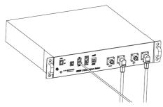
**Note:** if choosing lithium battery, make sure to connect the BMS communication cable between the battery and the inverter. You need to choose battery type as "lithium battery".
