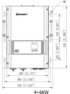
Install the unit by screwing the six setscrews.
