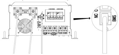
4. The other end of RJ45 insert to battery comm port.
