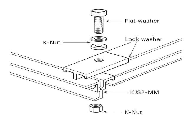
Slide a K-Nut into the deep channel of each rail section and rotate it flat to lock in place. Align the KJS2-MM joiner across the rail ends, ensuring proper positioning.
